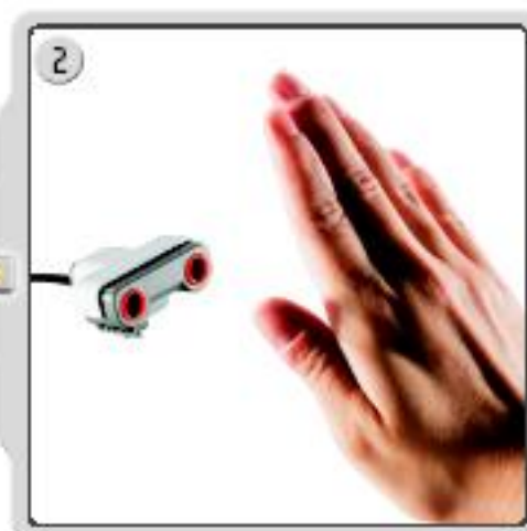
2 Measure the distance to an object. For example, move your hand closer to the sensor and watch the readings change.
